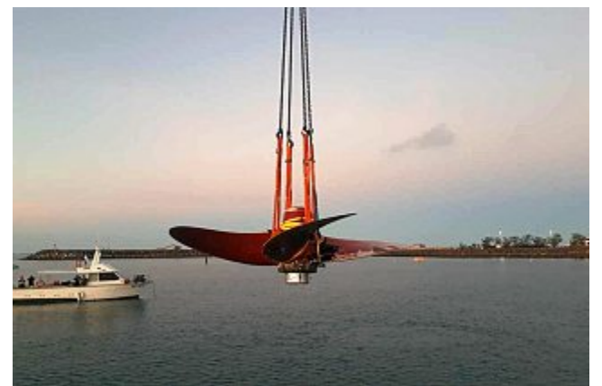
Subsea used a tugboat and gear such as lift bags and spreaders to bring the propeller to the surface. Photo: Ed Korber
